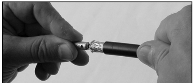
Figure 105: Deburring the Center Conductor
