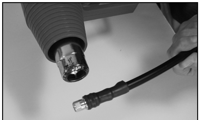
Figure 111: Applying the Heat Shrink Tubing
